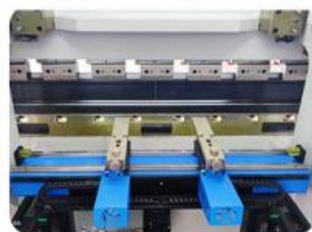
4 Axis Back Gauge (X,R,Z1,Z2)
