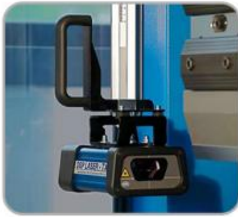
LASER Safety Guards
