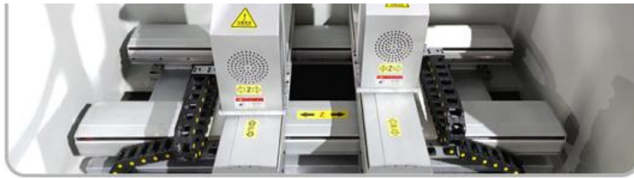
6 Axis Back Gauge (X1,X2,R1,R2,Z1,Z2)
