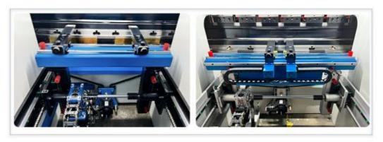
**Auto Crowing System:** To confrm a constant bend angle, manual or CNC crowning is essential which will offset potential deviations and allow for possible tooling wear to maintain parallel contacting surfaces. CNC crowning systems allow the press brake control to be pre-programmed with machine characteristics and defection data. Adjust the calculate and setting accordingly for different characteristics of different materials.
