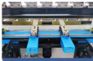
4 Axis Back Gauge (X,R,Z1,Z2)
