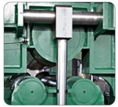
Release device :Hydraulic drop- end for easy removal of finished ferrule.
