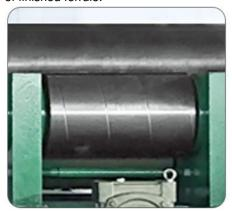
The top roller is designed as drum shape ,Bend a metal material into a perfect cylinder.
