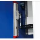
Linear Encoder Feedback The deformation is measured accurately and compensated
