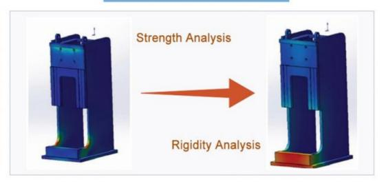
The key mechanical parts of the machine tool adopt finite element analysis to analyze the deformation and safety factor; so as to ensure the high rigidity requirements of the whole machine tool and the reliability of long-term use.
