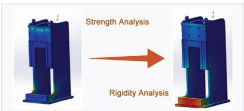
The key mechanical parts of the machine tool adopt finite element analysis to analyze the deformation and safety factor; so as to ensure the high rigidity requirements of the whole machine tool and the reliability of long-term use.
