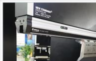
Auto Tool Clamping System WILA clamping system efficiently changes hydraulic and pneumatic tools
