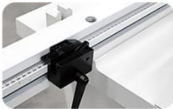
Vertical Adjustment and Front Stop Position Device
